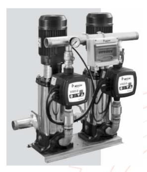
VSD.20- VLR is a booster set assembled with 2 VLR multistage centrifugal pumps and 2 VSD3 inverters. Designed to provide variable flow at constant pressure.
