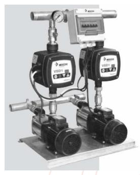
VSD.20- MULTINOX is a booster set assembled with 2 MULTINOX multi stage centrifugal pumps and 2 VSD1 or VSD1 Basic inverters. Designed to provide variable flow at constant pressure.
