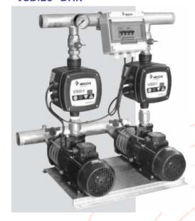
VSD.20- DHR is a booster set assembled with 2 DHR multistage centrifugal pumps and 2 VSD1 inverters. Designed to provide variable flow at constant pressure.
